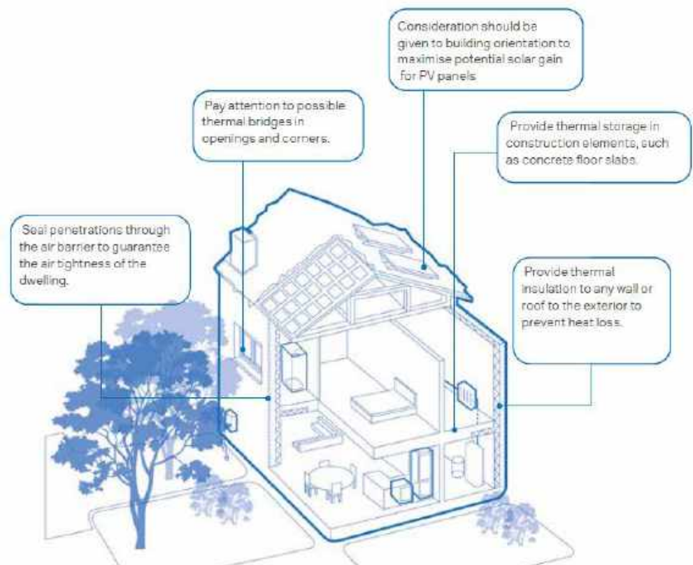
Figure 18. Diagram illustrating aspects relevant to energy efficient designs
